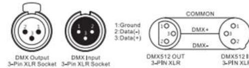
For installations where the DMX cable has to run a long distance or is in an electrically noisy enviroment, such as in a discotheque, it is recommended to use a DMX terminator. This helps in preventing corruption of the digital control signal by electrical noise. The DMX terminator is simply an XLR plug with a 120 Ω resistor connected between pins 2 and 3, which is then plugged into the output XLR socket of the last fixture in the chain. Please see illustrations
